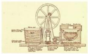
Jacob Perkin's Ice Machine (1834) (Closed cycle vapour compression refrigeration system with ethyl ether as the working fluid)
